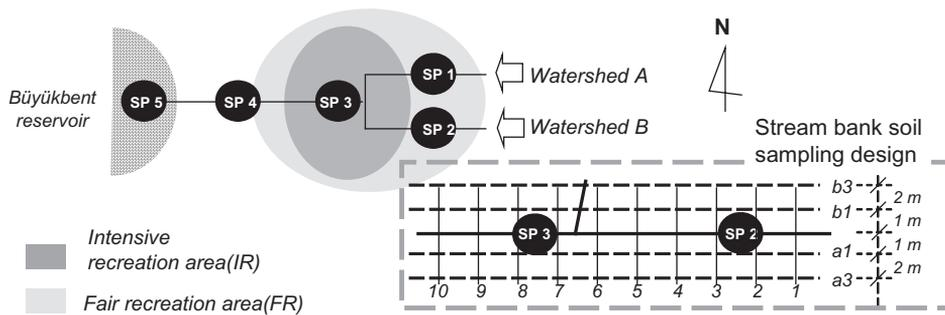
Fig. 2. Schematic representation of the water sampling points. Numbered black circles are water sampling points (SP 1, 2...5), and solid lines represent the creeks. The stream bank soil sampling points are taken on the transects (1, 2...10), 1 and 3 m away from the channel on both sides (a1, a3, b1, b3).
